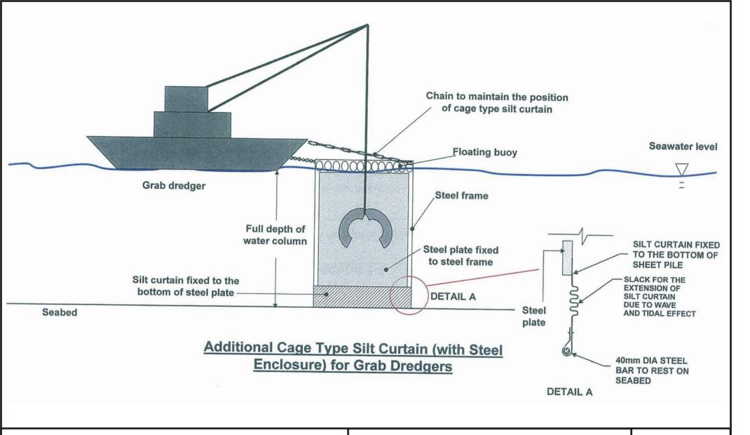
Figure 8 - Single layer of Cage Type silt curtain (with steel enclosure)
